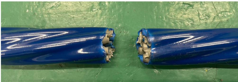
Coating adhesion kept after the break
