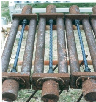
ECS after 7.5 years outdoor exposure under 70% GUTS tension in Okinawa
