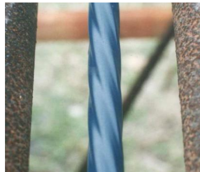
ECS after 7.5 years outdoor exposure under 70% GUTS tension in Okinawa
