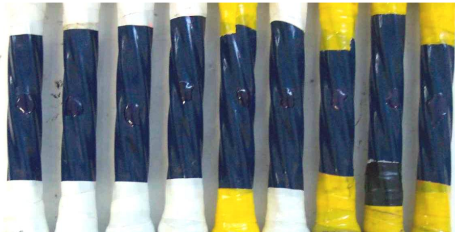
3,000 hour salt spray test for repair spots on artificial coating defects
