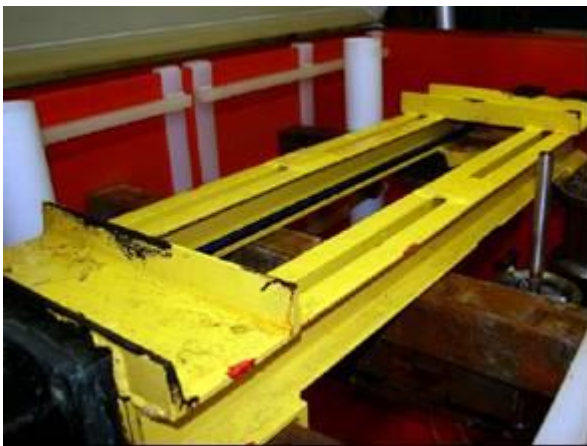
Salt spray (fog) test under 70% GUTS, 3000 hours
