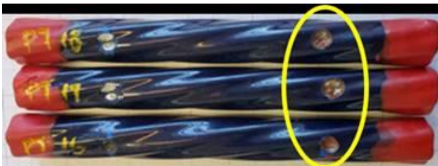
ECS samples with a hole after immersing into 3M CaCl 2 for 45days
