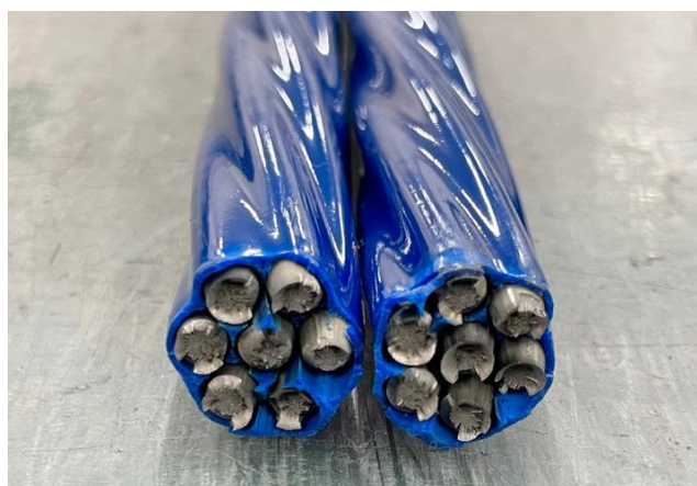
Ductile wire breaks
